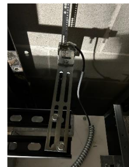
Figure 10: Sensor Mounting Plate Crosshead Installation
