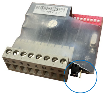
Figure 50: Non Terminated Hall Board
